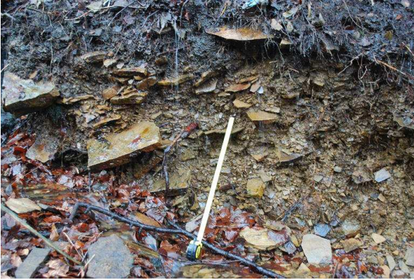
g) A jumble of sharp, angular fragments of sandstone mixed up with clay. The scale is 50cm long (Photo: Peter Kennett)
