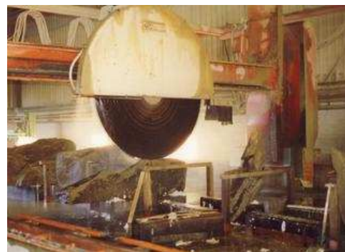
A 3m diameter rock saw cutting sandstone into uniform slabs (Johnsons Wellfield, Huddersfield. Photo: Peter Kennett)
