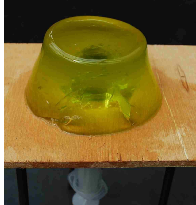
‘Cauldron subsidence’, after pulling the plunger back two or three times. A radial fracture can also be seen, produced when the plunger was pushed in again.
