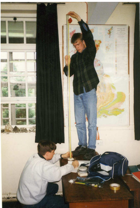
Students testing the rebound of a ball bearing from a rock sample (using a 2m long plastic tube)
