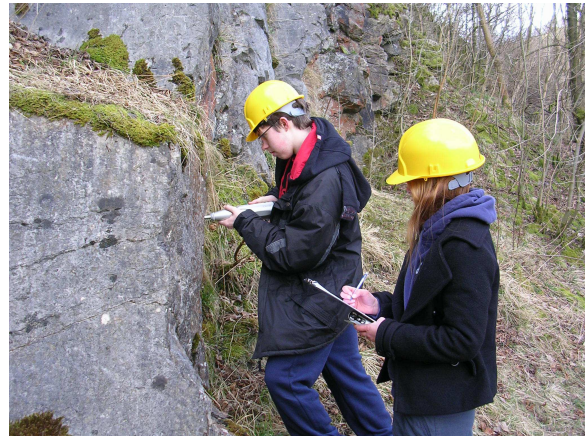
Students using a Schmidt Hammer to measure the strength of a limestone, as part of a tunnel planning exercise
