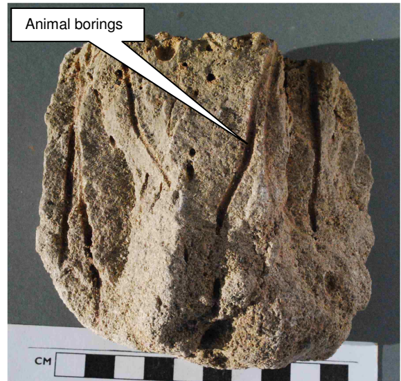
Photo 5: Side view of a hard limestone with tubes running through it. Lincolnshire Limestone, Jurassic, Ketton, England
