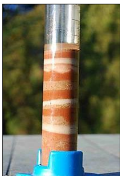
Beds in a sedimentary sequence in a measuring cylinder. (Peter Kennett).
