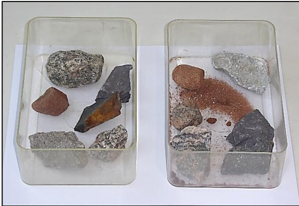
The trays – control on the left, 'freezer' tray on the right. (Chris King).
