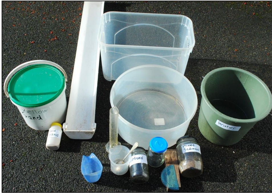
The apparatus and materials, consisting of: gutter with end stop; square plastic box; circular plastic box; measuring cylinder; scoop; beaker; dessert spoon; wood block; protractor; jar with lid; washed yellow sand in tub; washed red sand; mud in jar with lid; mixed sediment in jar with lid; bucket of water.
