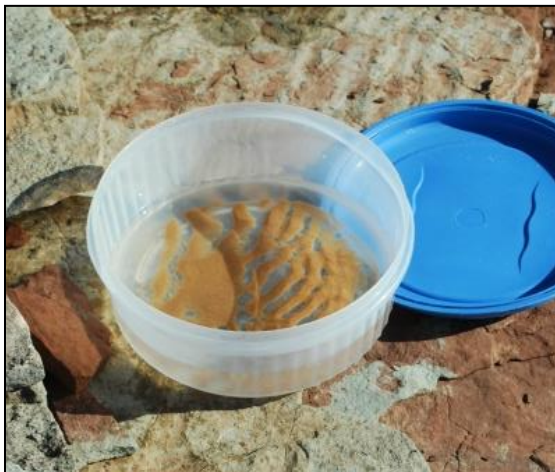
Symmetrical ripples (in a circular bowl, but a square one works better)
