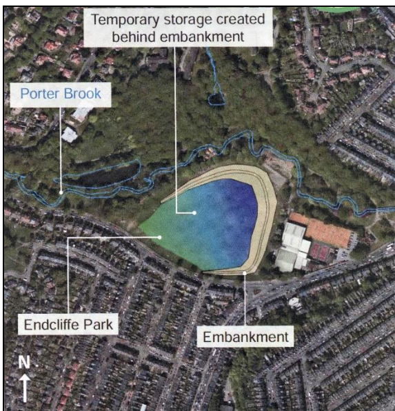
Plan showing potential location of the embankment and extent of temporary flood storage area created.
