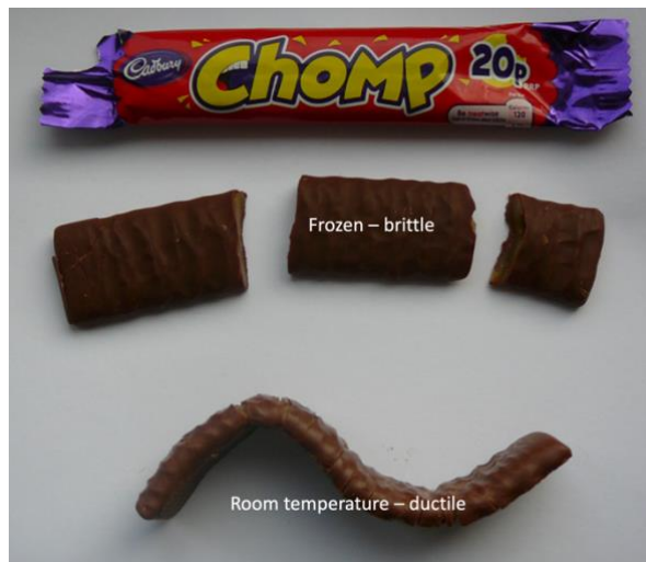
Figure 3: Chomp bars after same force was applied to them. (Pete Loader)
