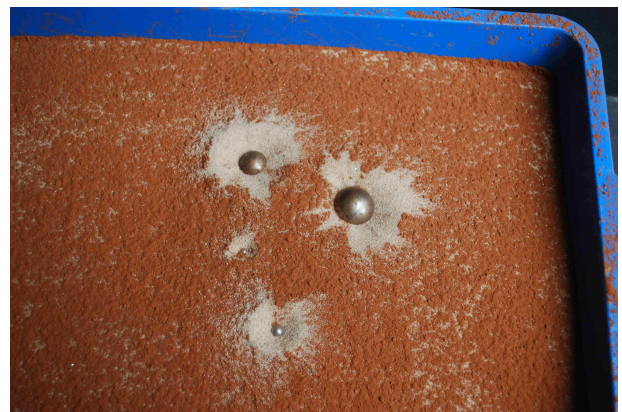
Craters produced by dropping 4 steel ball bearings of different sizes into a tray of sand (with a dusting of cocoa powder) (Photo: Peter Kennett)
