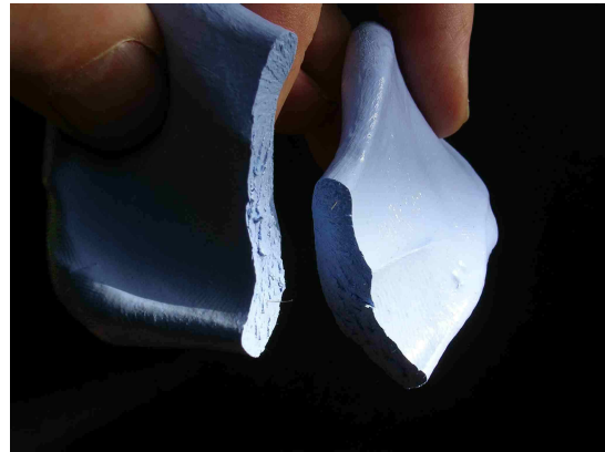
Brittle deformation when pulled apart
