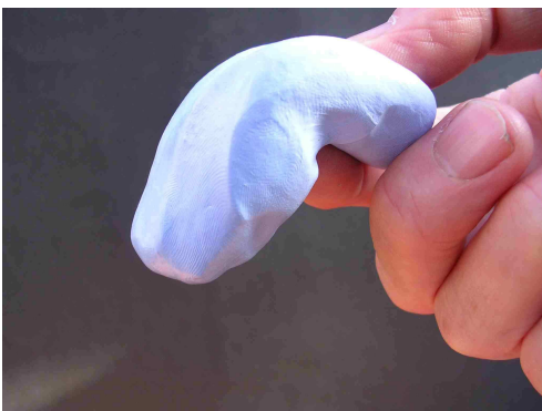
Plastic deformation under its own weight
