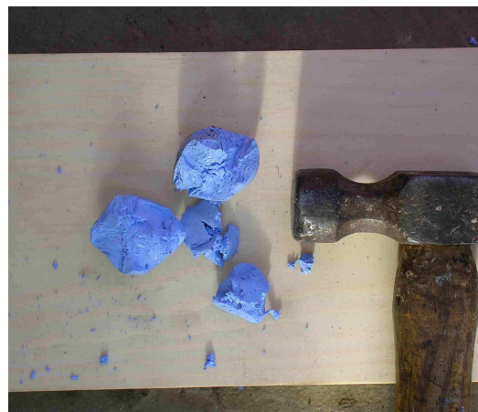
Brittle deformation when hit by a hammer (Photos: Peter Kennett)
