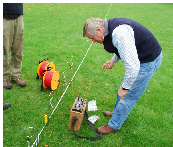
The way electrical methods are used in the field – in this case, to locate a buried steel drum (Photographs by Peter Kennett)
