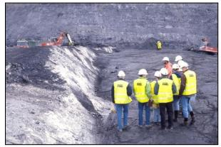
A steeply-inclined normal fault – formed by tensional forces pulling apart the rock mass, allowing the rocks on the right to slide downwards. Orgreave opencast site, South Yorkshire. © Peter Kennett, ESEU
