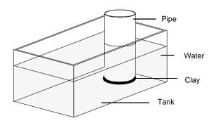
The demonstration is more effective if a circular ribbon of clay or Blu Tak<sup>TM</sup> is used as a seal between the pipe and the base of the tank – but this is not essential.
