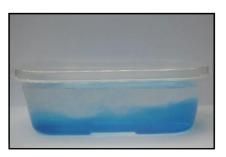
Iced water, coloured with blue food colouring, added to the left of the lunchbox – flowing along the bottom from left to right.
