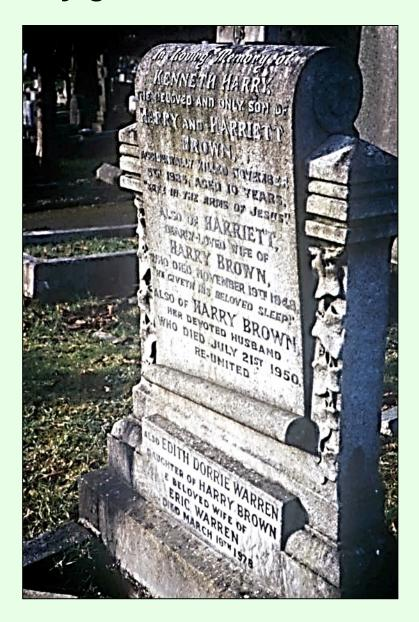
Marble, showing more weathering by carbonationsolution on the top surface than on the vertical surface, (shown by the lead letters standing further out from the marble on the top)
