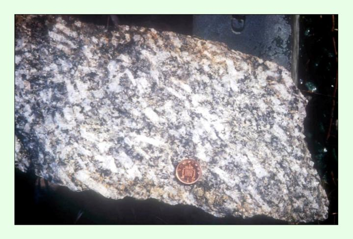
Chemical (oxidation) weathering, shown by orange discolouration on the edges of a broken Cornish granite
